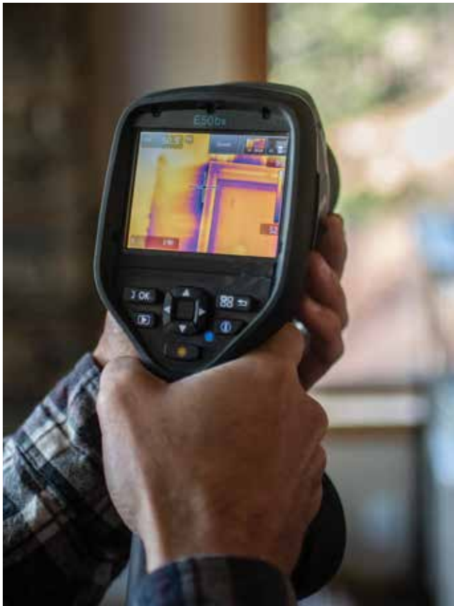
Paulson's thermal camera shows precisely where heat leaks from a home.
